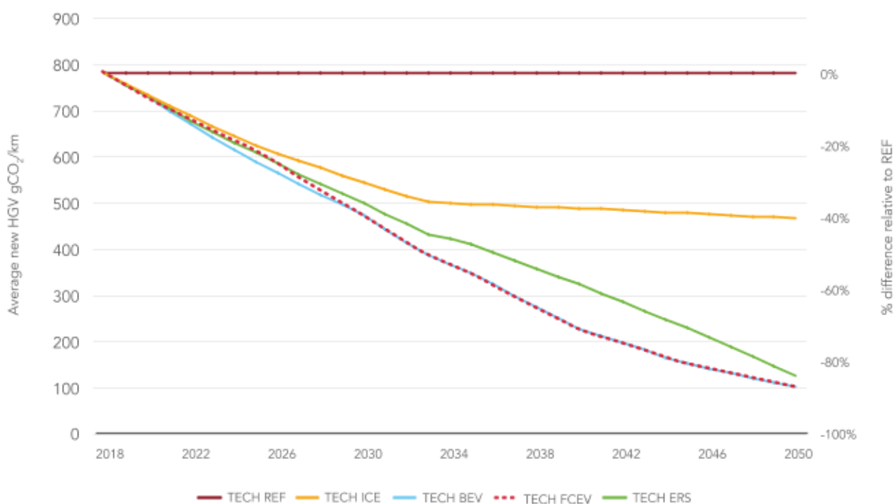
Figure 10. Impact of the ZEV scenarios on EU CO 2 emissions from the average new HGV in each scenario.
